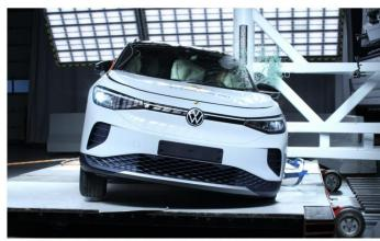
Crash and post-crash safety tests for batteries include complete vehicle tests, allowing structural as well as systemic protection systems to be proven (Courtesy of Polestar)
